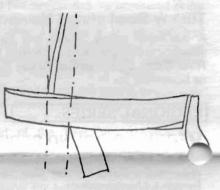
When we use the centerboard a little pulled in we also reduce turbulence in the centerboard box, since there is less empty space in it.
